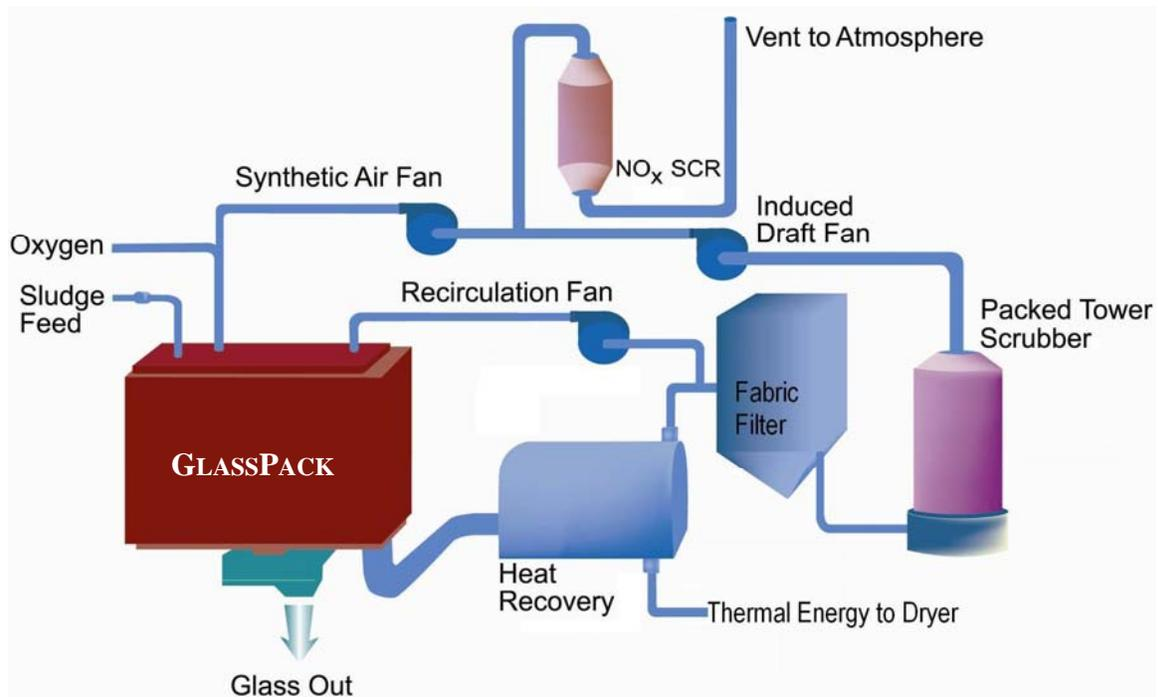
**Figure 2. GLASSPACK Closed-loop Oxygen Enhanced Combustion Configuration**
