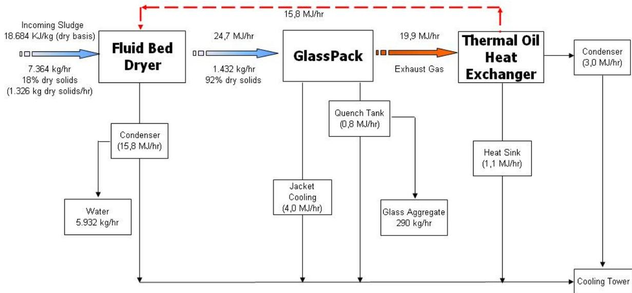
**Figure 4. Mass and energy balance for GlassPack installation at North Shore Sanitary District Sludge Recycling Facility, Zion, Illinois, USA.**
