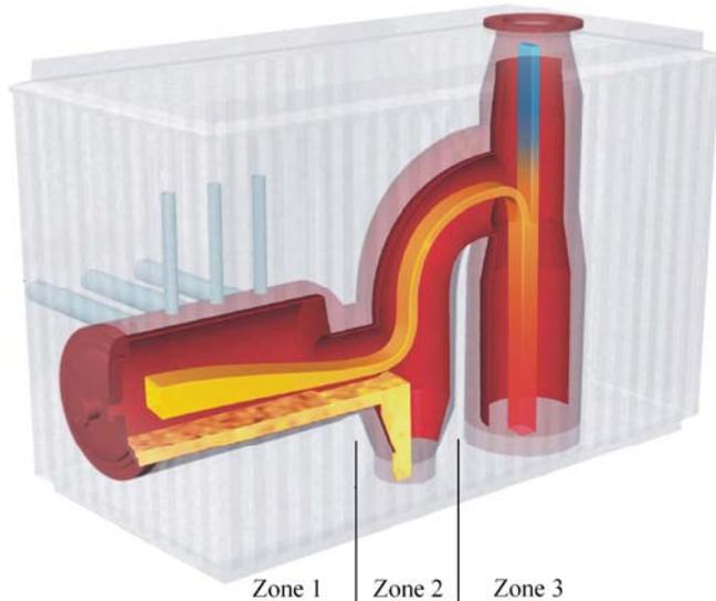
temperature are to eliminate expensive refractory-lined ductwork exterior to the melter, and to cool any particulate carryover below the softening point, thus eliminating ductwork fouling. The temperature of the Zone 3 exit gas varies depending on the temperature and quantity of the dilution gas, but is typically in the range of 370 ° to 870 ° C (700 ° to 1600 ° F) Higher temperature exit gas can provide for higher efficiencies in downstream heat recovery process.
