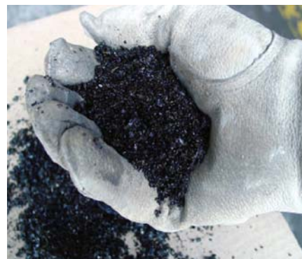
Glass aggregate product fresh from the quench tank.
