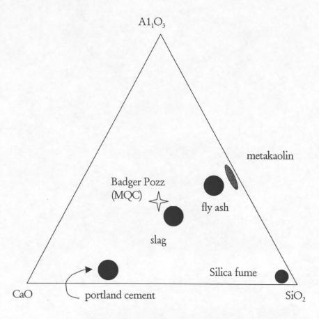
Figure 1. Ternary diagram showing typical oxide compositions of the cementitious and pozzolanic materials. The oxide composition of the Badger Pozz MQC material is closest to that of slag.
