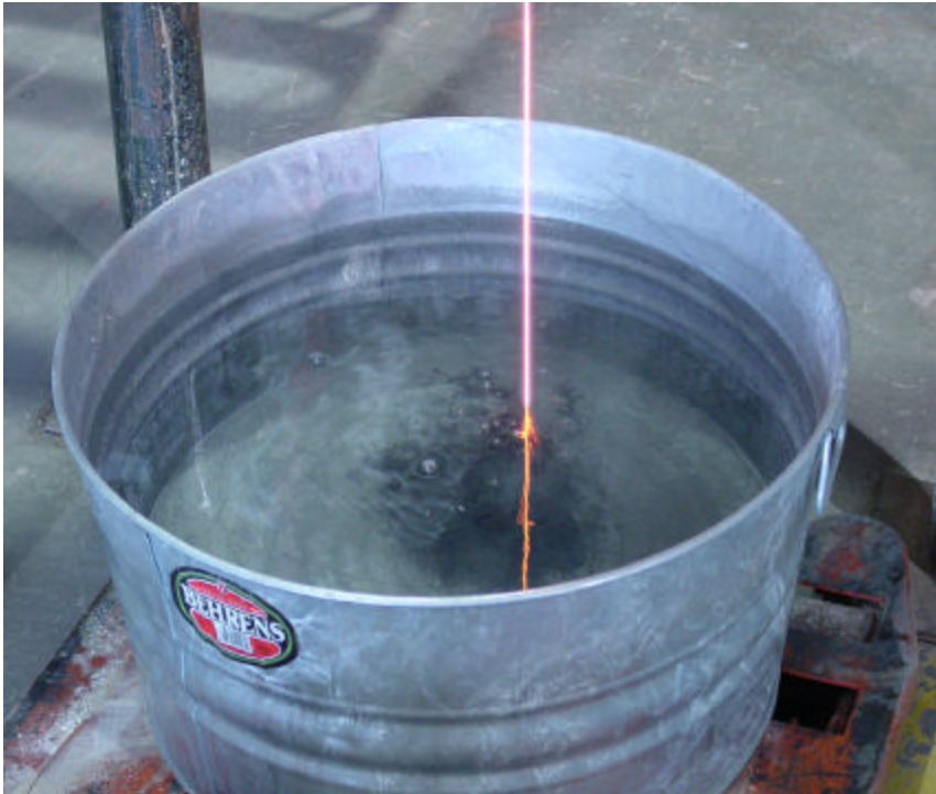
Water Quenching Molten Glass from Crucible Melt
