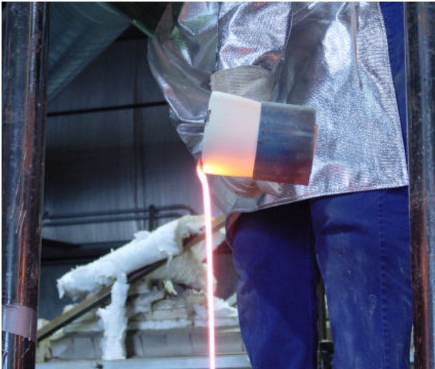
Pour-off of Molten Glass from Crucible
