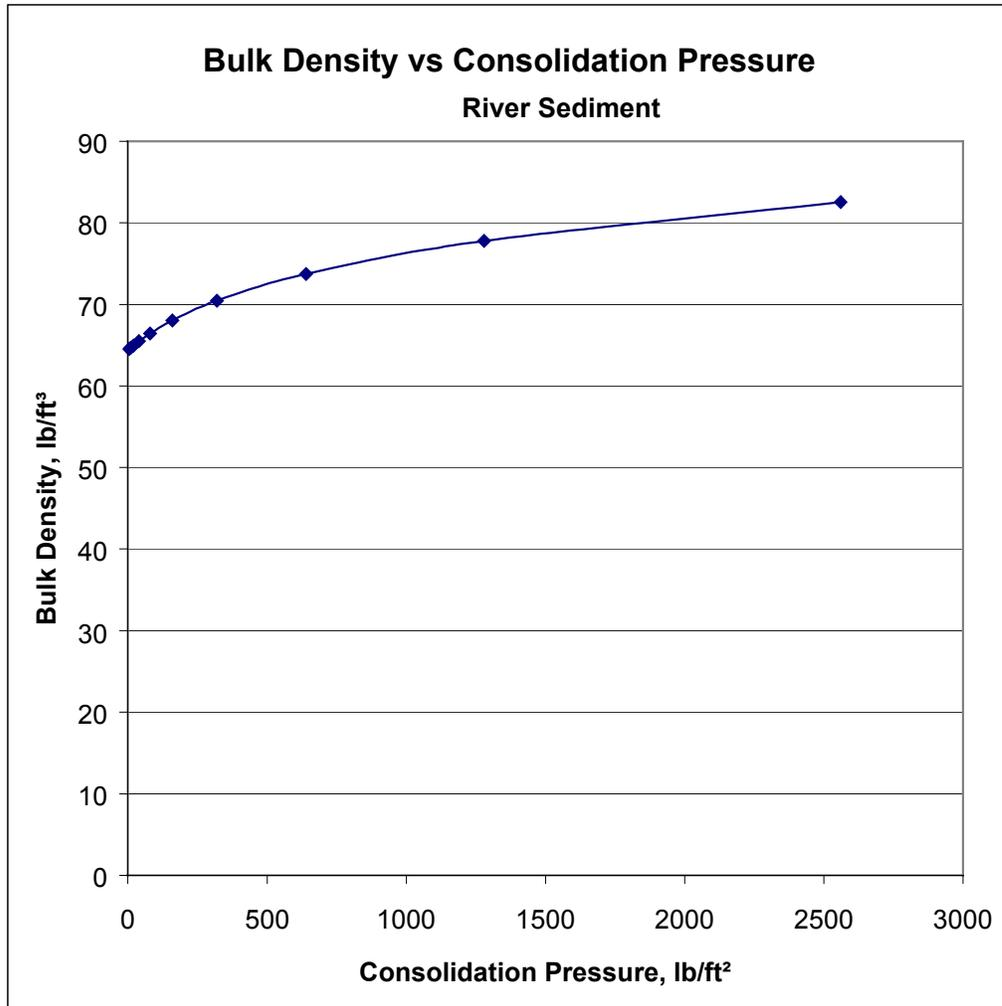
$$\text{Bulk Density} = \gamma = \gamma_0(1+(\sigma/\sigma_0))^B$$
