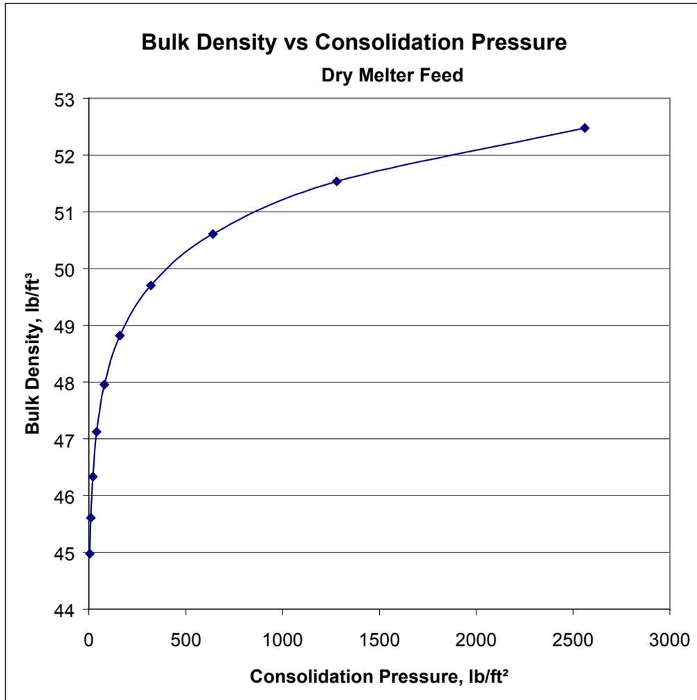
$$\text{Bulk Density} = \gamma = \gamma_0(1+(\sigma/\sigma_0))^\beta$$
