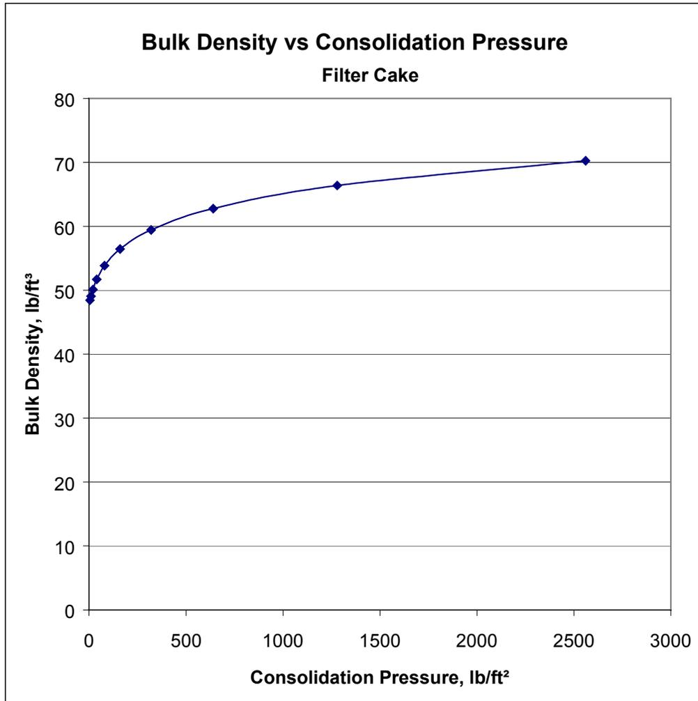
$$\text{Bulk Density} = \gamma = \gamma_0(1+(\sigma/\sigma_0))^B$$
