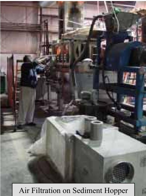
Air Filtration on Sediment Hopper
