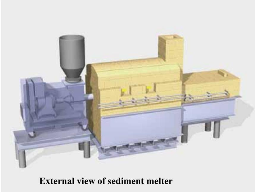
**External view of sediment melter**
