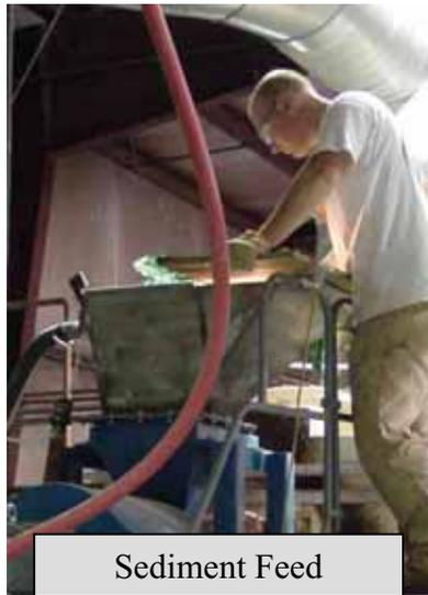
The moisture content of the river sediment affected feed rates. Moisture contents ranged from 5% to 20%. River sediment with higher moistures tended to bridge in the charger, and to cake around the auger. A technician permanently observed the feeding process, to make sure the charger was always feeding material to the melter.
