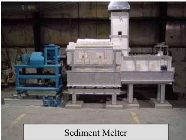
The melter evaluation was performed at Minergy's GlassPack Test Center in Winneconne, Wisconsin. A demonstration-scale melter was constructed, with operation of the melter from May to August, 2001. The pilot program was designed to confirm that the technology can destroy PCB contamination, stabilize trace metals, and convert the mineral content of river sediment
