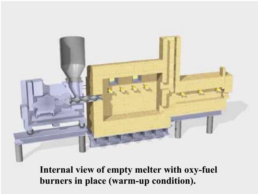
**Internal view of empty melter with oxy-fuel burners in place (warm-up condition).****Introduction to Glass Furnaces**
